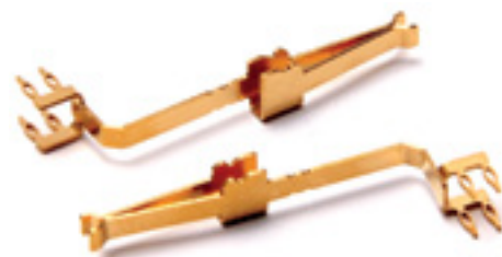
.012" Thick Beryllium Copper Contact Springs. Photoetched Blank. Die Formed. Heat Treated. Gold Plated.
