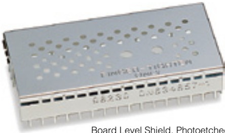
Board Level Shield. Photoetched Blank. Cover: .010" Thick FH Brass Die Formed. Fence: .015" Thick 1/2H Brass. Depth Etched Bend Lines. Hand Formed. Solder Corner. Tin Plated.
